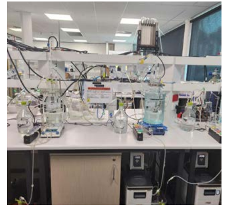
Lab simulation of field conditions for MIC testing
